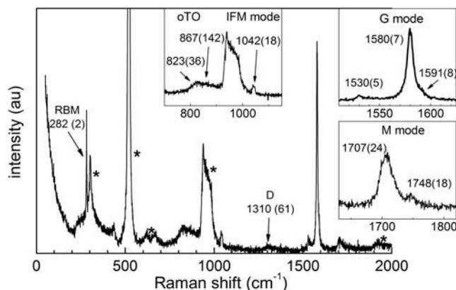
**Figure 2** Measured Raman spectrum from individual semiconducting SWNT. Seven bands are observed: RBM, two intermediate frequency, D, G, M and G'. The peak wave numbers are shown together with full width half maxima (FWHM) of various features taken in parentheses. Asterix indicates Si-substrate peaks.
