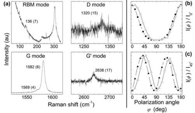
**Figure 4** a) Experimental Raman spectrum from one light spot on individual DWNT sample for laser excitation energy  $EL = 1.92 \text{ eV}$ . Four bands are observed: RBM, D, G and G'. The peak wave numbers are shown (with FWHM in parentheses); normalized intensity  $I(\varphi)/I(0)$  angular  $\varphi$  dependence of G mode of SWNT (open symbols) and DWNT (full symbols) in two configurations: VV (b) and VH (c).
