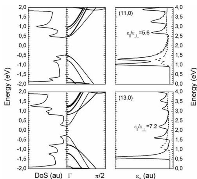
**Figure 5** Density of states, band structure and dielectric function of selected semiconducting single-wall carbon nanotubes. Dotted line denotes  $\epsilon_2$  perpendicular to the nanotube axis and solid line denotes  $\epsilon_2$  parallel to the nanotube axis.
