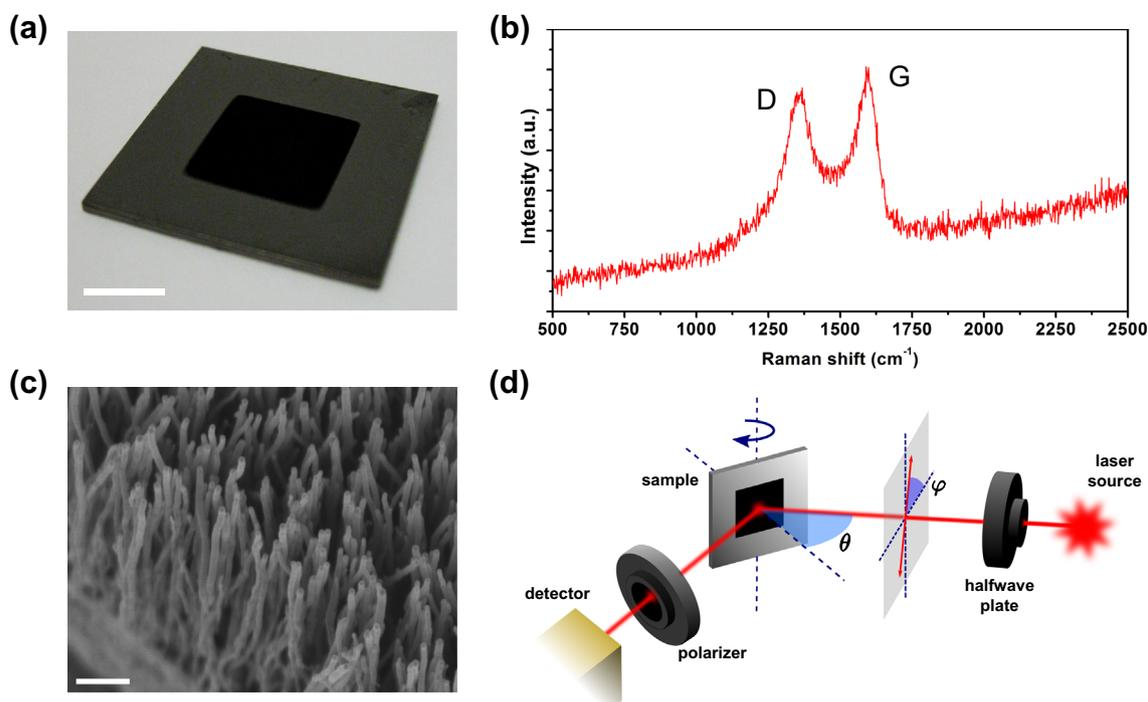
**Fig. 1** – (a) Real photograph of the sample, the scale bar equal to 5 mm. (b) Raman spectrum of MWCNTs forming the array (laser line 514 nm). (c) SEM image of the array, the scale bar equal to 300 nm. (d) Experimental setup for the reflectance measurements.
