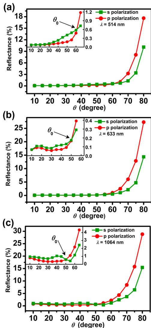
**Fig. 2 – Specular reflectance for different incidence angles for s- and p-polarized incoming light with three radiation wavelengths: 514 nm (a), 633 nm (b) and 1064 nm (c). Insets show the range of low  $\theta$  angles with  $\theta_0$  indicated for each wavelength.**
