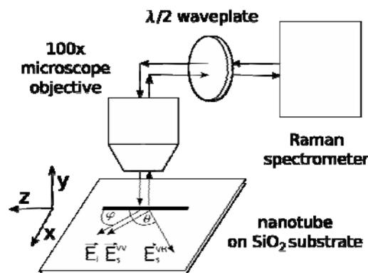
**Figure 1** The electric vector  $E_{i(s)}$  of the light incident (scattered) from the Y direction forms an angle  $\varphi$  ( $\theta = \varphi$  for VV or  $\theta = \varphi + \pi/2$  for VH configuration) with the nanotube axis, oriented along the Z direction. In particular, VH configuration with  $\varphi = 0$  is denoted as Y(XZ)Y or in the simplified notation (XZ). A half-wave ( $\lambda/2$ ) retardation plate is used to change the angle  $\varphi$ .
