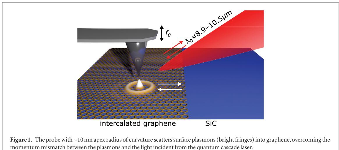
**Figure 1.** The probe with  $\sim 10$  nm apex radius of curvature scatters surface plasmons (bright fringes) into graphene, overcoming the momentum mismatch between the plasmons and the light incident from the quantum cascade laser.
